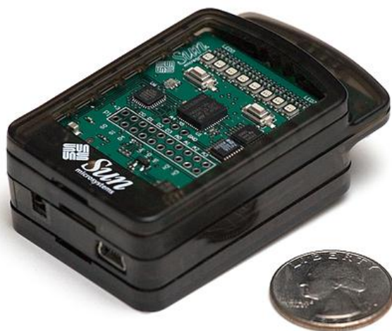
FIGURE 5-1: SUN SPOT NODE (IMAGE CREDIT: SUN MICROSYSTEMS)
